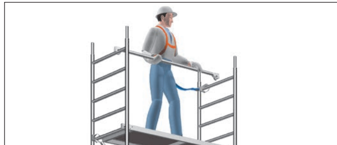
Fig. 3: Safe fitting of guardrails with PSA
