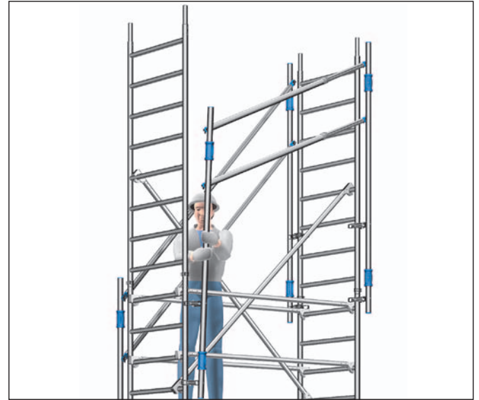
Fig. 5: Upward movement of the advance guardrail system
