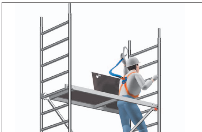
Fig. 1: Attachment of PSA during ascent onto the unsecured level
