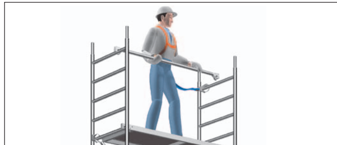
Fig. 3: Safe assembly of rear guardrails using PSA
