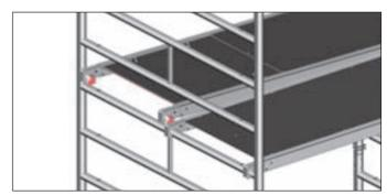
The red locking clips of the decks permit effortless installation and removal by a single person; first open them and place the deck with the opened clips on the rung, then open the opposite clips and lift out the deck
