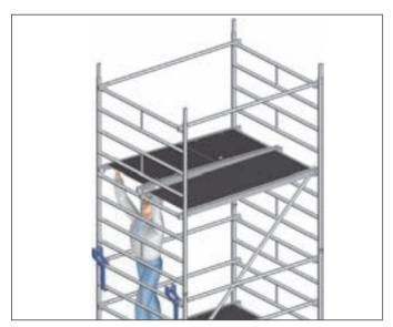
**4.** Insert diagonal braces 12, access deck 19 and deck 18. The diagonal braces must be installed in a tower-like (zig-zag) form on both sides.
