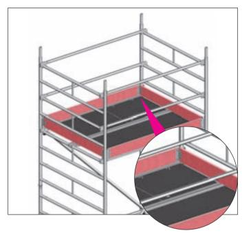
**1.** To complete the working platform, attach toe boards with claw 17 and end toe boards 16.
