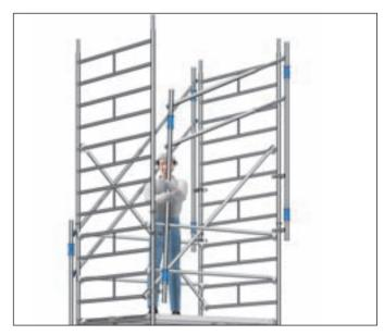
Fig. 5: Upward movement of the advance guardrail system
