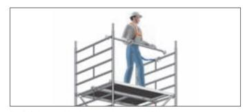
Fig. 3: Safe assembly of rear guardrails using PSA
