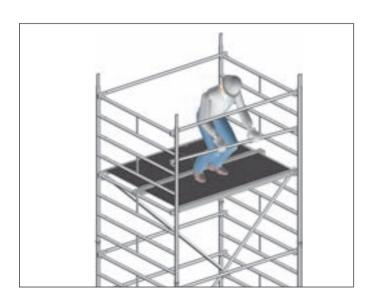
**5.** Climb up to the next level and fit additional rear guardrails 8 to the second rung above the platform surface.
